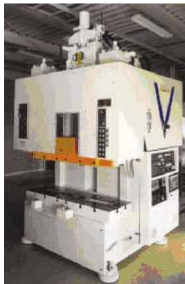
The PIM System, which combines several technologies to enable insert molding.
