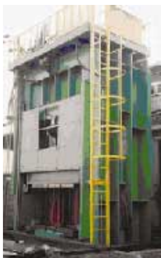
Advanced Material's 3,000 ton press. The company also has 300, 500, and 1,000 ton presses that can be adapted for various materials and uses.
