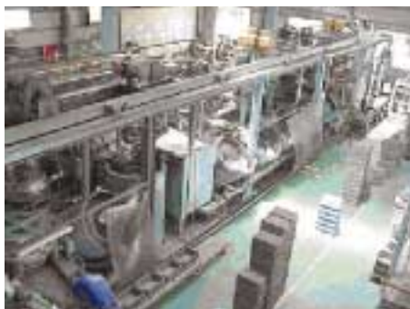
The washing process is essential to create clean-looking screws that Okitsu Rasen is proud of.
